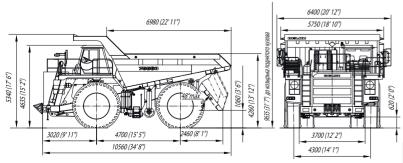
\*Overall dimensions are specified for standard equipping of the dump truck
